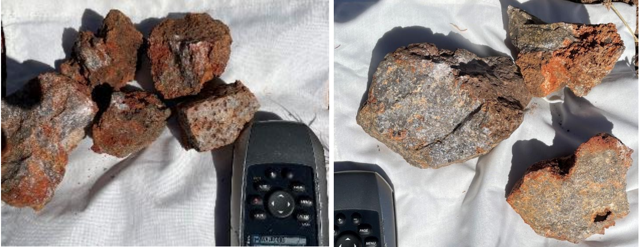
Figure 12: LHS WALR0003 iron rich black quartzite? with voids - 0.27g/t Au from South Wallaby; RHS WALR0007 siliceous intergranular quartzite? - 0.43g/t Au from Central Wallaby
