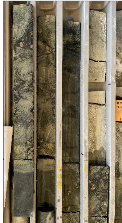
Figure 11: EVDD2203 – 101m - Breccia infill mineralisation
