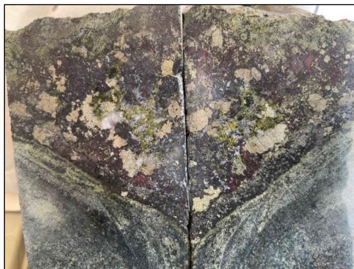
Figure 1: Sphalerite mineralisation in altered amphibolite showing epidote carbonate alteration and replacement by pyrite – EVDD2203 – 110.5m
