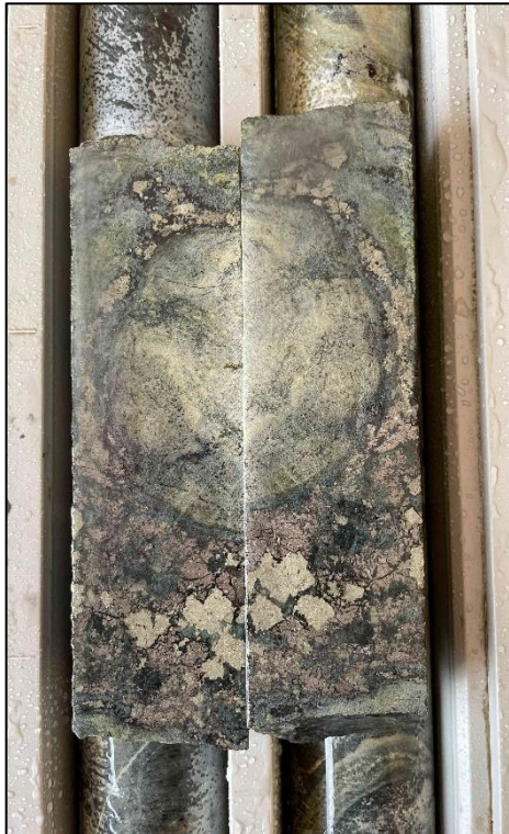
Figure 9: EVDD2201 – 75.9m Breccia clast showing sphalerite infill mineralisation over printed by coarse pyrite
